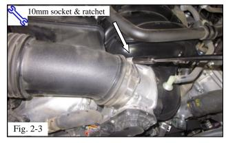
(c) Loosen the inlet tube hose clamp at the throttle body (Fig. 2-3).
