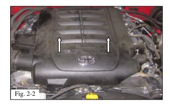
(b) Lift up on the front of the engine cover and pull forward to remove it (Fig. 2-2).
