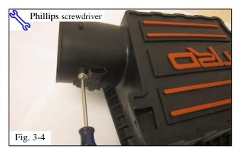
(e) Install the mass airflow sensor into the TRD air cleaner lid (Fig. 3-4).
