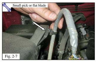
(g) Unclip the mass airflow sensor wiring harness from the side of the factory air cleaner lid (Fig. 2-7). Use a small pick or flat blade to depress the clip tangs.
