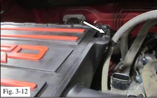
(o) Attach the mass air flow wire harness to the TRD air cleaner lid (Fig. 3-12).
