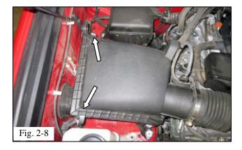
(h) Unclip the two (2) retaining clips on the air cleaner lid and remove the complete upper assembly (Fig. 2-8).
