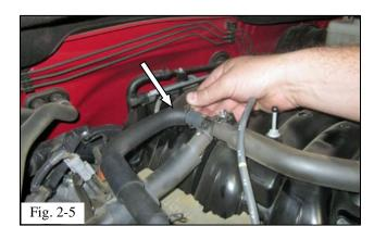
(e) Squeeze the clamp on the other end of the PCV hose and disconnect it from the "T" junction (Fig. 2-5).
