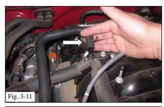
(n) Connect the other end of the PCV hose to the "T" junction with the second spring clamp removed in step 2(1) (Fig 3-11).
